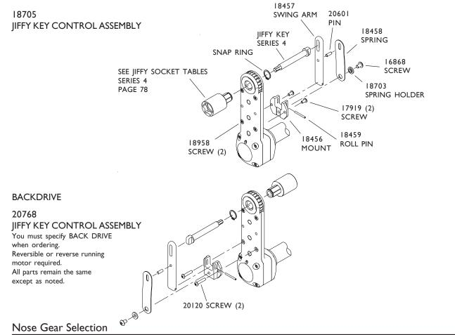
The SOCKET DRIVER will adapt the attachment to accept Series 4 Sockets starting on Page 78. Order with or without the
